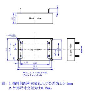
Notes: 1. The tolerance of pin spacing and installation hole's dimension is  $\pm 0.1$  mm.
