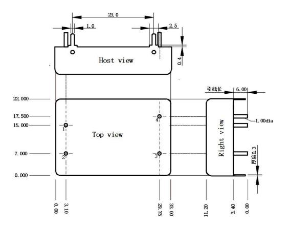
Note:  $1_{x}$  The tolerance of needle diameter and between two pins is  $\pm 0.1$ mm;
