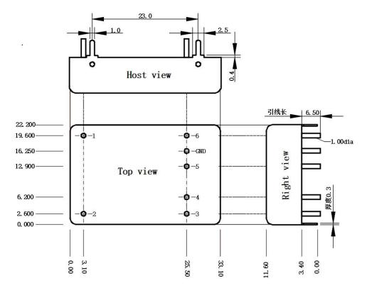
Note: 1. The tolerance of needle diameter and between two pins is  $\pm 0.1$ mm;
