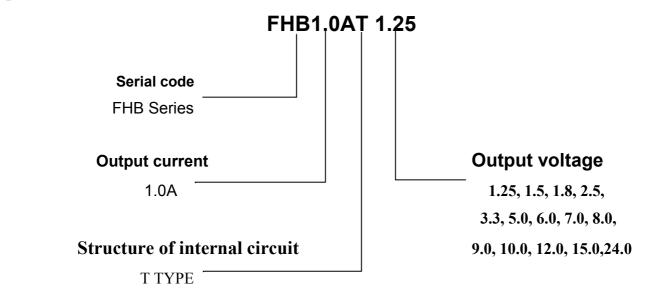
1.0A High Temperature Step Down DC-DC Power Converters
