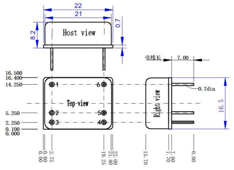
Note: 1. The tolerance of needle diameter and between two pins is  $\pm 0.1$  mm; 2. The tolerance of external dimension is  $\pm 0.2$  mm
