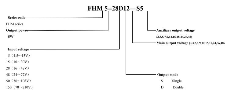
Note: "—" in the above model means isolation, that is input is always isolated from output, so the first "—" is required. If the main output is not isolated from the auxiliary output, there is no the second "—". There will be no —SAOUT, if there is no the auxiliary output.
