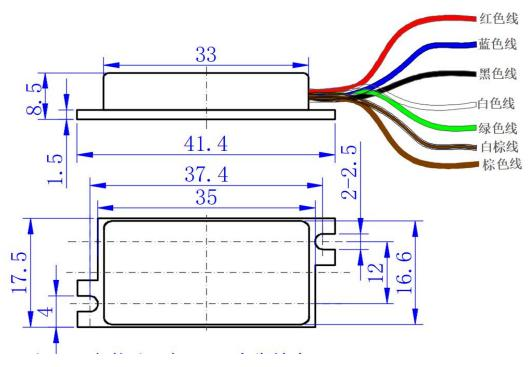
Note: 1  $\times$  Mounting hole and mounting hole spacing dimension tolerance is  $\pm 0.1 \mathrm{mm}$
