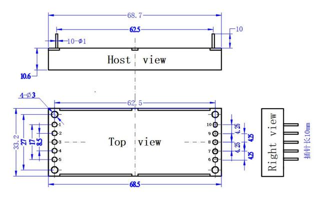
Note: 1. The tolerance of needle diameter and between two pins is  $\pm 0.1$ mm; 2. The tolerance of external dimension is  $\pm 0.2$ mm
