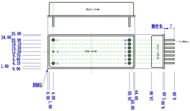
Note: 1. The tolerance of needle diameter and between two pins is  $\pm 0.1$ mm;
