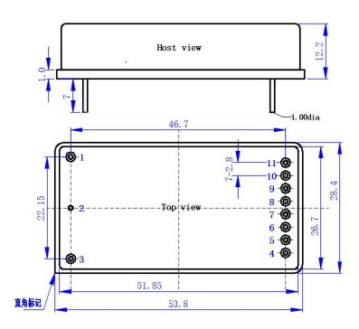
Note: 1. The tolerance of needle diameter and between two pins is  $\pm 0.1$ mm;
