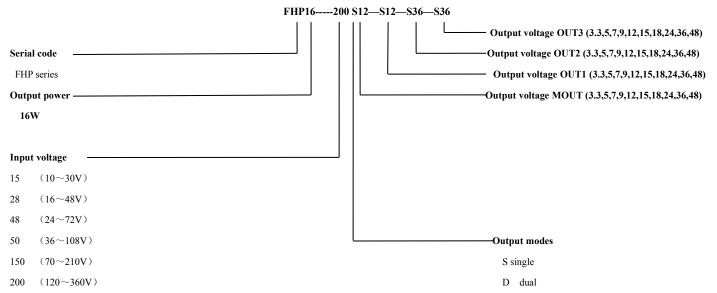
NOTE: "—" in model refers to the meaning of isolation. It is always isolated between input and output. For this reason, the first "-" is necessary. The later three "-" may not appear. S\*\*\* can also be represented with D\*\*\*or S\*\*\*S\*\*\*. There are at most four S\*\*\* in a model. D\*\*\* represents two S\*\*\*.
