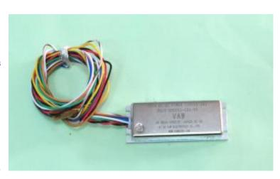
18W Watt, High Temperature DC-DC Power Converters
