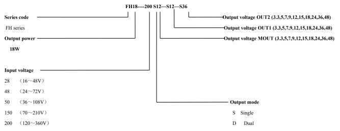
NOTE: "—" in model refers to the meaning of isolation. If the single output is adopted, there is no—SOUT1—SOUT2; if dual output is adopted, there is no—SOUT2.
