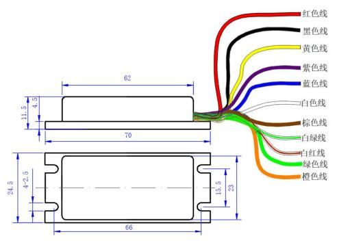
Note: 1. Mounting hole and mounting hole spacing dimension tolerance is  $\pm 0.1$ mm
