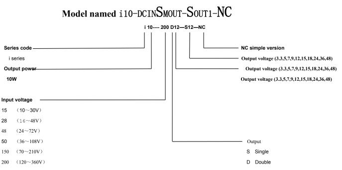
Note: "—" in the above model means isolation, that is input is always isolated from output, so the first "—" is required. The following "—" may not appear, which means no isolation or there is isolation between outputs. S\*\*\* can also be  $D^{***}$   $\mathfrak{R}$  S\*\*\*S\*\*\*. There are three S\*\*\* at most in a model. D\*\*\* means two S\*\*\*.
