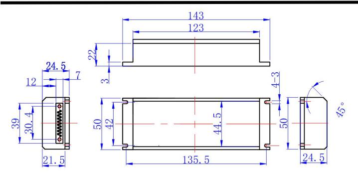
Note: 1. Mounting hole and mounting hole spacing dimension tolerance is  $\pm 0.1$ mm 2. The tolerance of external dimension is  $\pm 0.2$ mm
