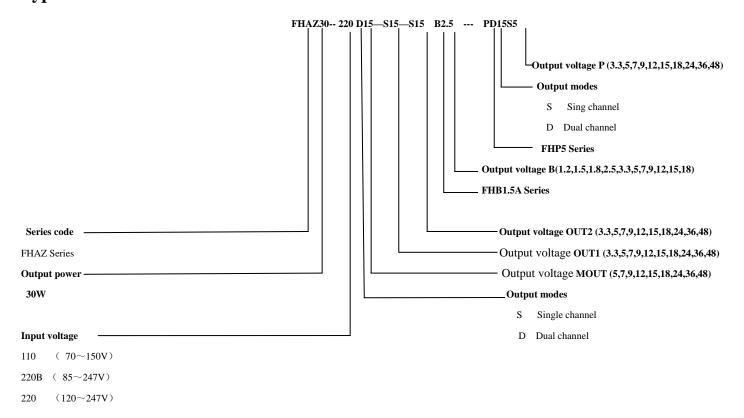
NOTE: "—" in model refers to the meaning of isolation. If the master output is single channel, there is no—SOUT1—SOUT2; if it is double channel, there is no -SOUT2. When FHB1.5A and FHP5 are connected to the output of a channel, then its model will be represented with the output it closes to. If the channel connected to FHB1.5A and FHP5 is not introduced, then it is marked with -B or NP.
