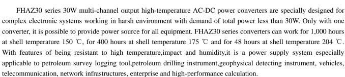
FHAZ30 series converters have three alternative input ranges including AC 70~150V(frequency 0Hz~400Hz), AC85~247V(frequency 0Hz~400Hz) and AC210~247V(frequency 0Hz~400Hz). It provides more than 10 channels of output and output can provide five isolated GNDs at most. They can be connected to form different output combinations as per requirement. Within the entire temperature range and conversion between full load and no-load, the output voltage fluctuation is within 2%.
